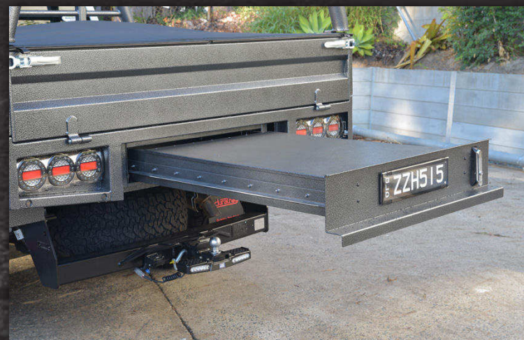
Rolla-drawer integrated into tail light panel
