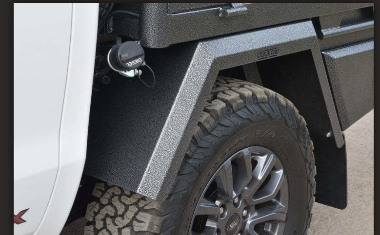
One piece laser cut flared mudguards
