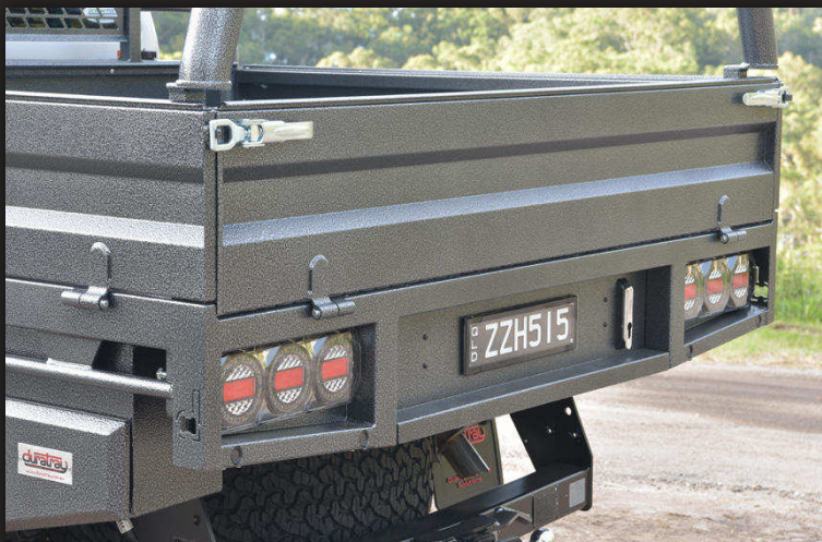
Recessed full width tail light panel Optional integrated roll-drawer & LED Maxilamp tail lights
