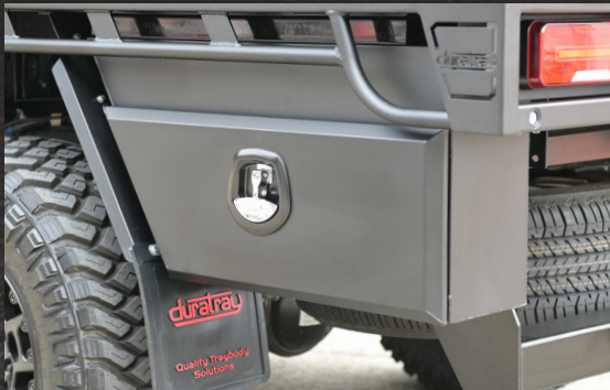
Under body toolboxes, colour coded
