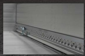
Tie down track with adjustable eyelets Integrated into inside of dropsides
